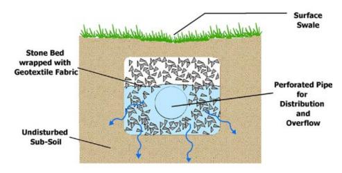
Infiltration trench with perforated pipe (UIC)
